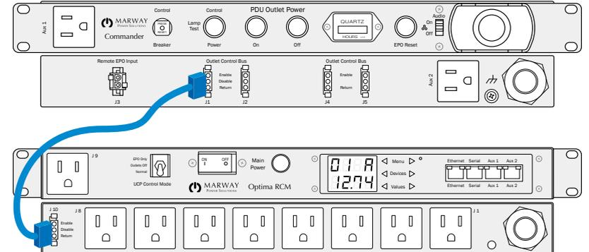
(up) position. The switch name and position labels may be different. Additionally, pins 2 & 3 on the PDU's EPO connector must be jumpered.
