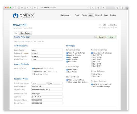
access to a PDU, the assignment of explicit permissions uniquely to each user allows for more control. The exact available permissions may vary based on the available features of any given PDU model.
