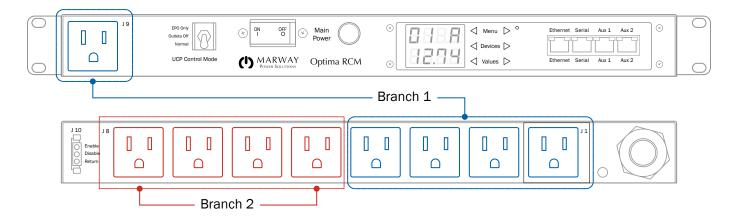
For Group 6 units with 5-15R outlets, each breaker branch is rated for 12/15 A. Any one outlet can carry a continuous load up to 12 Amps (with no draw on other outlets), or a combination of outlets on one branch can draw a total of up to 12 Amps. The total for the whole PDU is 24 amps (the rating of the inlet connector, which happens to coincide withe the sum of the branches).
