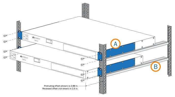
Note the illustration is conceptual, and not intended to depict any specific model, chassis size, or exact bracket hole pattern.
