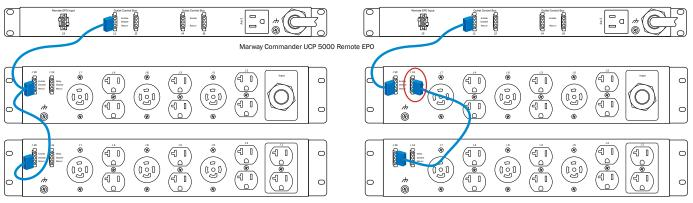
Using the "Enable" connectors, each PDU receives the On signal at the same time.
