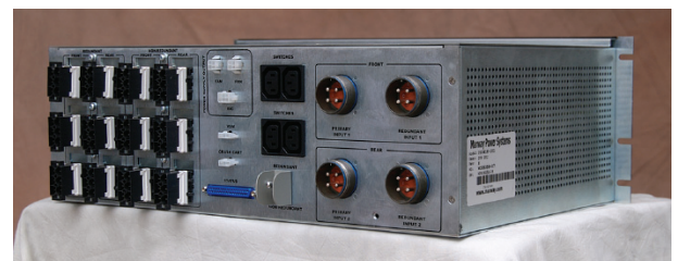
This unit served as the power center for a blade server farm which used 208 VAC input to provide AC as well as 12 and 48 VDC output. It includes on-board redundant power inputs with 13ms auto transfer, extensive signal monitoring, and remote control. MIL-SPEC connectors saved space for what had to be a compact design.
