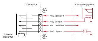
Shown is conceptually what's inside the UCP, and a simplified example of how to use the J4 and J5 connectors for auxiliary Power On signals.
