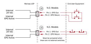
This diagram shows conceptually what's inside the UCP, and how to use the J3 connector to attach one or more external EPO buttons.
